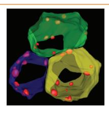
Delicate  $\gamma$ -Fe<sub>2</sub>O<sub>3</sub> @ macroporous silica composites with well-dispersed small  $\gamma$ -Fe<sub>2</sub>O<sub>3</sub> nanoparticles and open pore networks are fabricated as efficient arsenic adsorbents. Electron tomography technique confirms that iron oxide nanoparticles are spatially separated and anchored on the pore walls. Spatially well-dispersed small nanoparticles and open pore networks make composites promising for both As (III) and As (V) removal.
