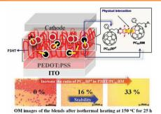
A new  $PC_{61}BM$ -based fullerene, [6,6]-phenyl- $C_{61}$  butyric acid pentafluorophenyl ester ( $PC_{61}BP^F$ ) is presented. Supramolecular attraction between the pentafluorophenyl group of  $PC_{61}BP^F$  and the  $C_{60}$  cores of  $PC_{61}BP^F/PC_{61}BM$  can effectively suppress the n-type  $PC_{61}BP^F/PC_{61}BM$  materials from severe aggregation to mitigate the morphological evolution and preserve the device performance.
