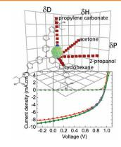
The binary solvent gradient method is used to determine the Hansen solubility parameters (HSP) of a star-shaped D- $\pi$ -A small molecule and a fullerene derivative. The HSPs are used to predict suitable green formulations to successfully replace halogenated solvents in solution-processed active layer in bulk heterojunction photovoltaic devices.
