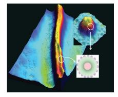
The doped molecules inside a dendritic box control 32 molecular rotors on the surface of the dendrimer and trigger chain-reaction of supramolecular structures, nanometer to milli-meter scale by harnessing electrical or optical energy. The communication pathway between molecular rotor, dendritic core molecule, and the dendrimer is identified as a non-chemical route for programming giant supramolecular architectures via molecular programming.
