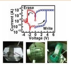
The first reprogrammable sticker-type organic memory is successfully demonstrated. The erasable sticker-type organic memory with a ready-to-conduct graphene electrode underlying can be easily molded onto arbitrary substrates and functions normally. It is believed that the newly designed sticker-type organic memory with reprogrammable feature may greatly broaden organic memory applications and advantage for the development of future soft electronic systems.
