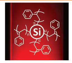
Highly luminescent, solution processable silicon nanocrystals/polystyrene hybrid materials are synthesized using size-independent radical-initiated hydrosilylation. Combining the properties of nanocrystals with polymer significantly increases solubility and processability, provides the opportunity to fabricate uniform nano- and microscale architectures, and renders silicon particles chemically resistant to prolonged exposure to strongly basic conditions.
